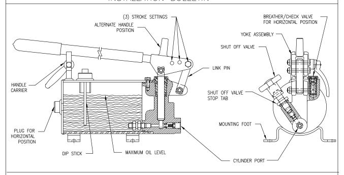
THE PRINCE HANDPUMP IS DESIGNED FOR EITHER HORIZONTAL OR VERTICAL MOUNTING.
