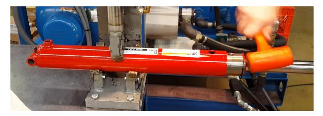
Now, use the special pliers to once again compress the snap ring and tap it past the tip of the tube until the snap ring seats in the groove. Visually confirm the snap ring is in place by confirming the presence of a gap between the open ends of the snap ring.
