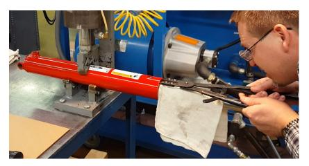
Using a dead blow hammer, tap on a cross bar until the snap ring pops out.
