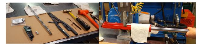
After placing cloths over the ports to absorb remaining oil, slowly pull the rod until the piston touches the gland.
