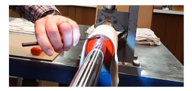
Protect the rod from possible dings or dents, then insert the pliers into the snap ring holes and compress the snap ring.
