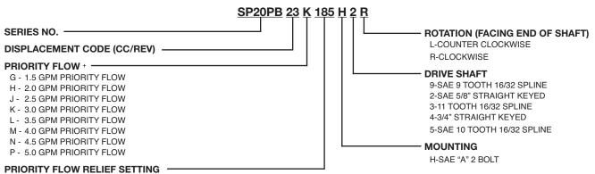
THE THREE DIGIT CODE REPRESENTS RELIEF VALVE SETTING DIVIDED BY 10. FOR INSTANCE A CODE NUMBER OF 185 REPRESENTS A RELIEF SETTING OF 1850 PSI. (RELIEF SETTING MUST BE BETWEEN 1000 AND 2250 PSI.)
