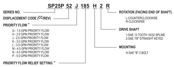
THE THREE DIGIT CODE REPRESENTS RELIEF VALVE SETTING DIVIDED BY 10. FOR INSTANCE A CODE NUMBER OF 185 REPRESENTS A FULL FLOW RELIEF SETTING OF 1850 PSI. (RELIEF SETTING MUST BE BETWEEN 1000 AND 2250 PSI.)
