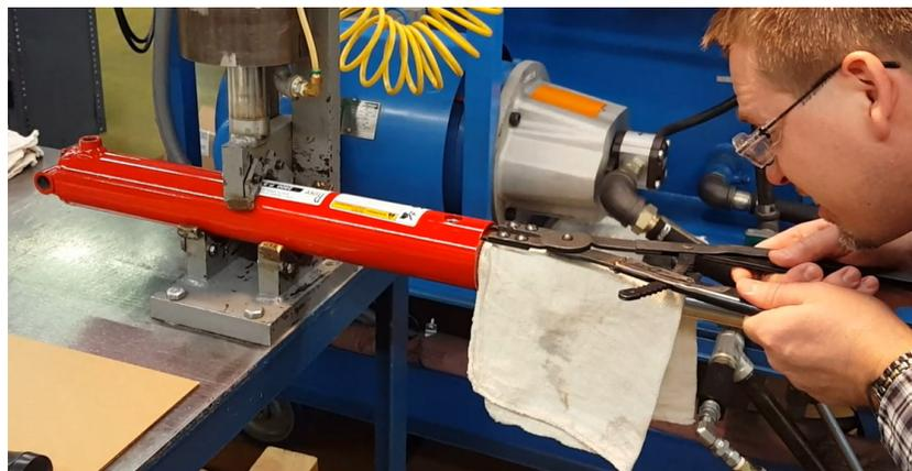
Using a dead blow hammer, tap on a cross bar until the snap ring pops out.
