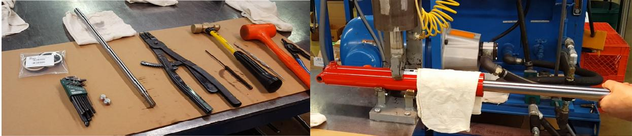
After placing cloths over the ports to absorb remaining oil, slowly pull the rod until the piston touches the gland.
