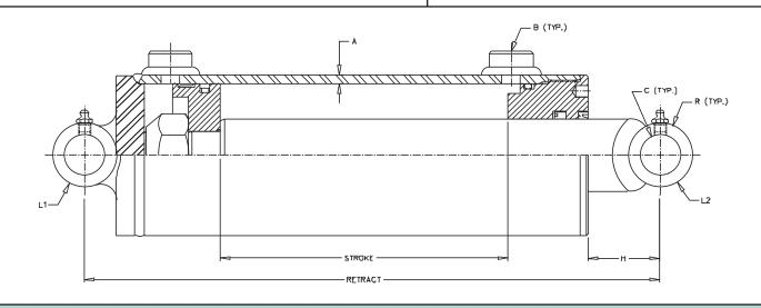
Rods are sized for a maximum safe push load (2:1 safety factor) given in the table. This is based on the pin configuration shown with no center support. Recommended pin material 100,000 PSI minimum yield strength
