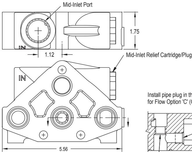
Section can be converted from C to S, or S to C, prior to installing section in the stack valve assy.
