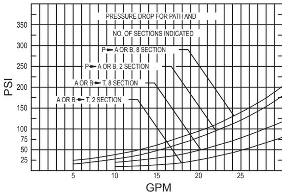
Oil 140 SUS at 110 degrees F. The pressure drop curves are representative, but the actual pressure drop will vary some from valve to valve. More detailed test data is available upon request.
