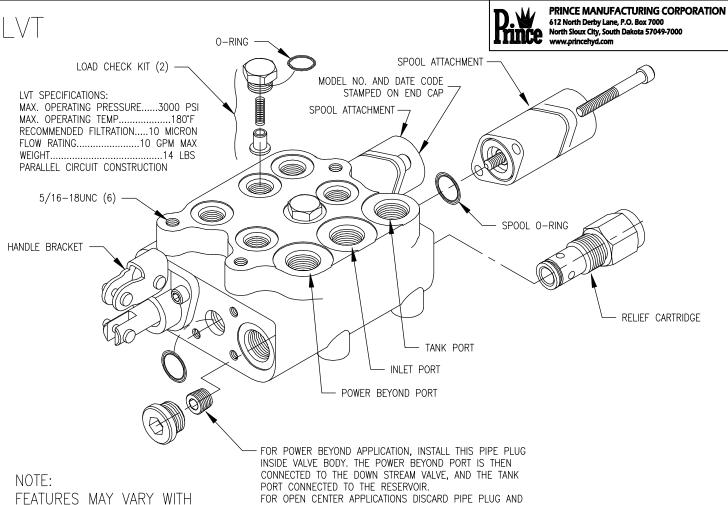
MODEL NO. CONSULT CATALOG PARTS MANUAL AVAILABLE AT www.princehyd.com PUT A STEEL PLUG IN POWER BEYOND PORT. FOR CLOSED CENTER APPLICATIONS, INSTALL PIPE PLUG AND PUT A STEEL PLUG IN THE POWER BEYOND PORT.
