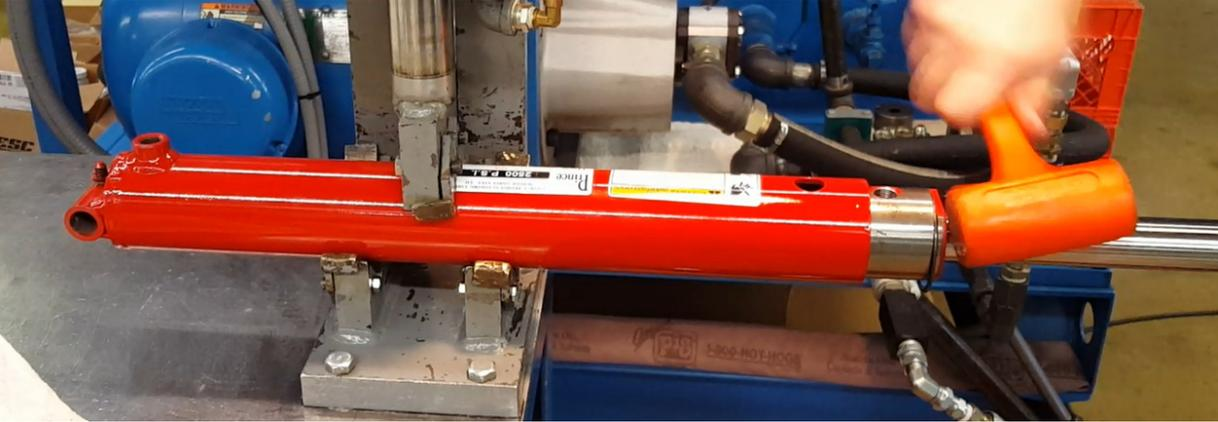
Now, use the special pliers to once again compress the snap ring and tap it past the tip of the tube until the snap ring seats in the groove. Visually confirm the snap ring is in place by confirming the presence of a gap between the open ends of the snap ring.
