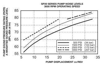
Pump acoustical data was determined in accordance with ANSI/B93.71M. Hydraulic fluid power-Pumps-Test code for the determination of airborne noise levels
