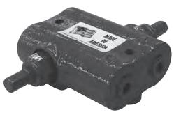
The PRINCE valve model DRV is a differential poppet type double relief. This valve uses the same relief cartridge as the model RV. The double relief is used in systems that require cross over relief protection such as reversible hydraulic motor, or double acting cylinders.
