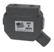
The PRINCE model RD-400 is a constant volume priority divider. It can be used in applications where two circuits are to be supplied by a single pump such as power steering systems. In operation the flow of oil supplied to the inlet is divided into two flows, the priority flow and the excess flow. The priority flow will remain nearly constant with variations in pressure on either the priority or excess flow port and will also remain nearly constant with variations in the inlet flow.
